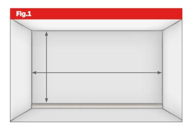
Measure, mark and cut horizontal strips for top and bottom. Apply bead of adhesive to back of panel strips and offer into position (Fig 2). Check level using spirit level and secure in position using nail gun. NB before proceeding, please check for any cables and pipes using a detector.
