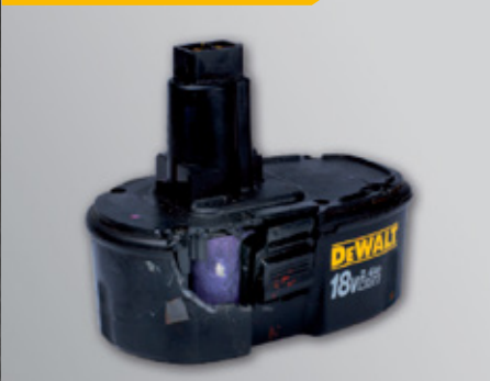
User dropped battery causing severe damage
