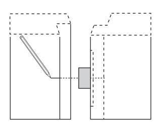
Position the latch receiver plate over the marked centre line. Align drill holes for fixing screws with the centre line. Mark around plate on the top rebate section.
