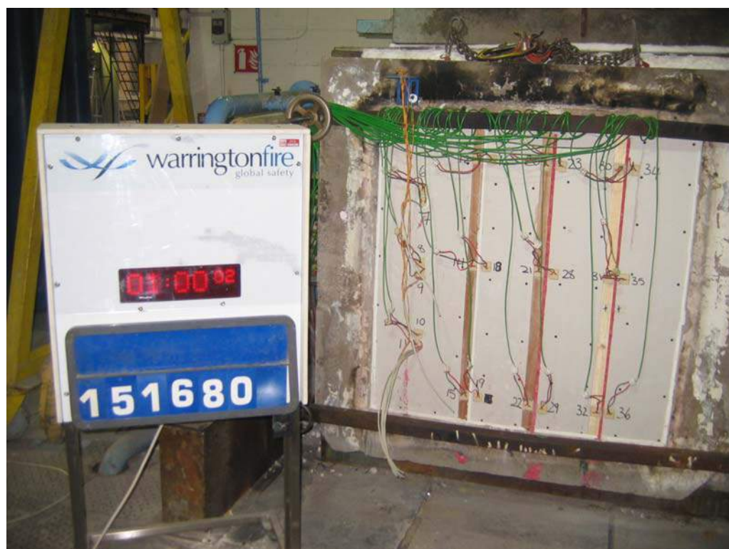
The unexposed face of the construction after 60 minutes of testing
