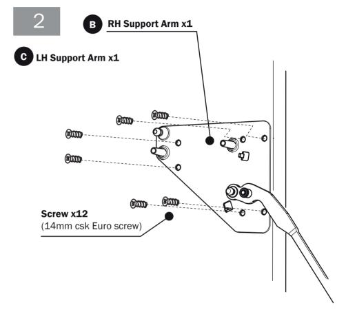
Lift the support arm & press piston onto the bracket pins.
