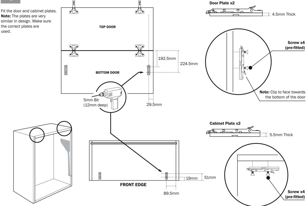
Fit the door assembly to the unit 6 aligning the hinge and bracket arms with plates. Clip into place.
